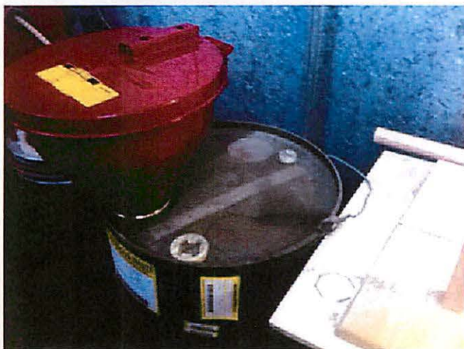
Item #7 threaded and latched funnel on hazardous waste drum.
