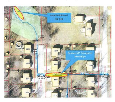
Later in April, while connecting the basin outflow pipes to the existing storm piping system, staff found piping between the properties at 2205 and 2209 to be significantly deteriorated and damaged. This damage was not evident at the time the study and design were completed by WRS in 2017. Due to the location of this pipe, the condition, and the construction left to complete the project, it was determined that replacement of the pipe is necessary.
