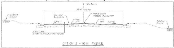
This option has an estimated cost of \$903,220 with an estimated life of 5-7 years. In lieu of using pavement fabric to control reflective cracking, the asphalt overlay is sawcut (and sealed) to match the existing concrete pavement joint pattern. This allows the asphalt overlay to "move" with the concrete pavement and prevents random reflective cracking. The sawcuts are sealed to prevent water from entering the joints.
