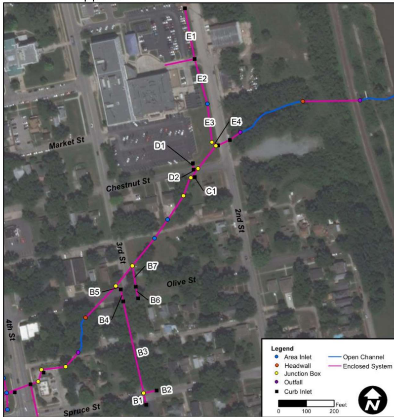
Figure 62: Existing Lateral System Hydraulic Routing Map
