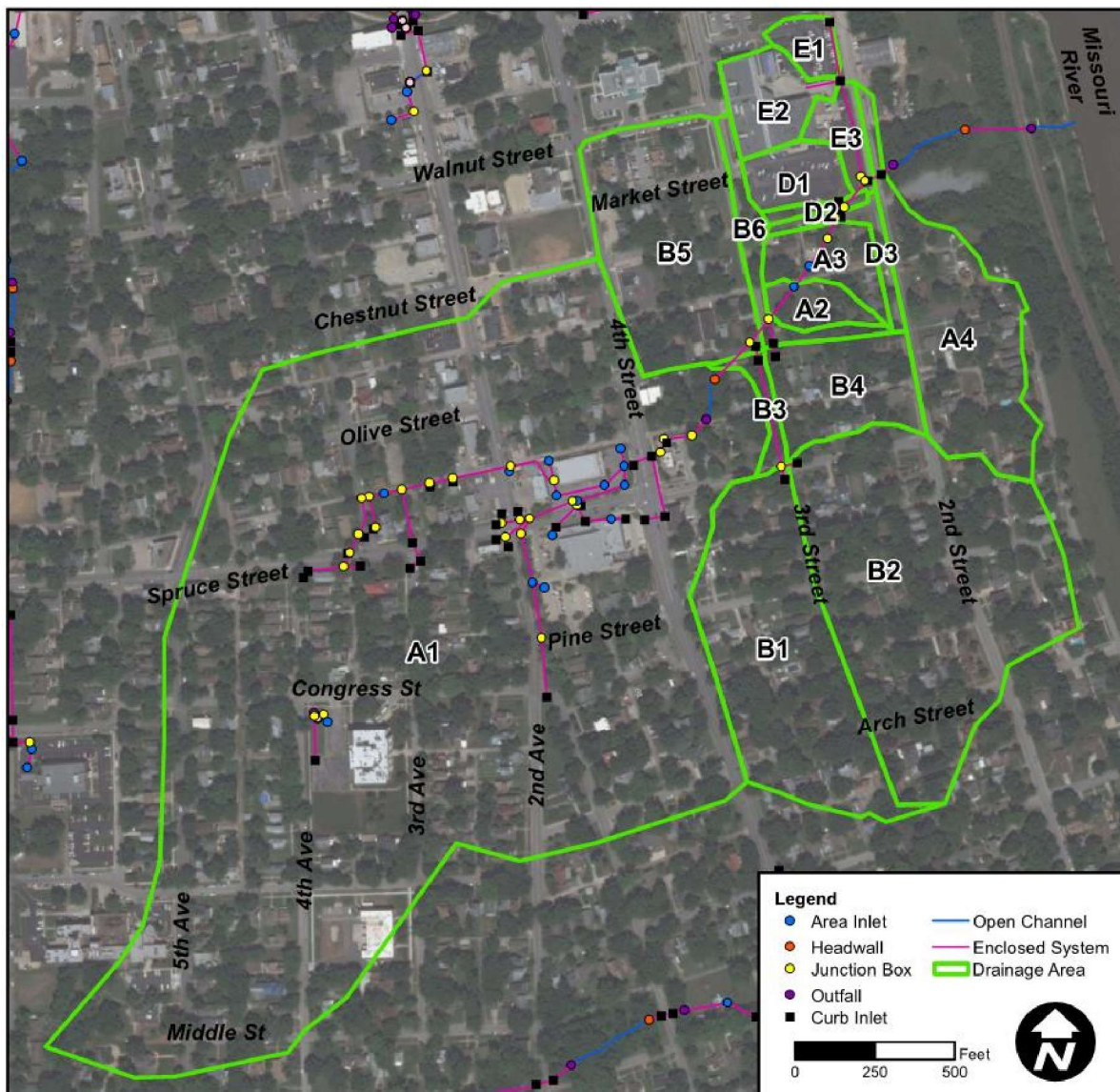
Figure 9: Drainage Area and Hydrologic Routing Map
