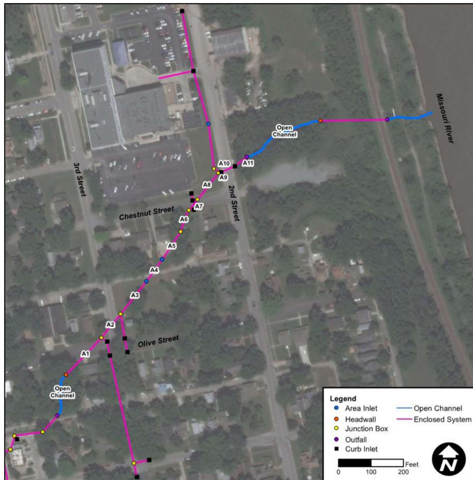
Figure 10: Existing Main System Hydraulic Routing Map
