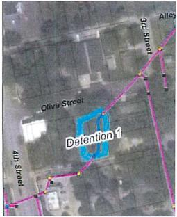
The report indicates that a detention basin (Option 1) at this location is not large enough to be effective. Option 2 creates a "Bio-Swale" to improve the quality of surface water that enters the storm drainage system from lower intensity storms similar to those installed in 700 block of Ottawa Street and in the Stubby Park stormwater project. Option 3 would essentially recreate the existing situation at the conclusion of the project.
